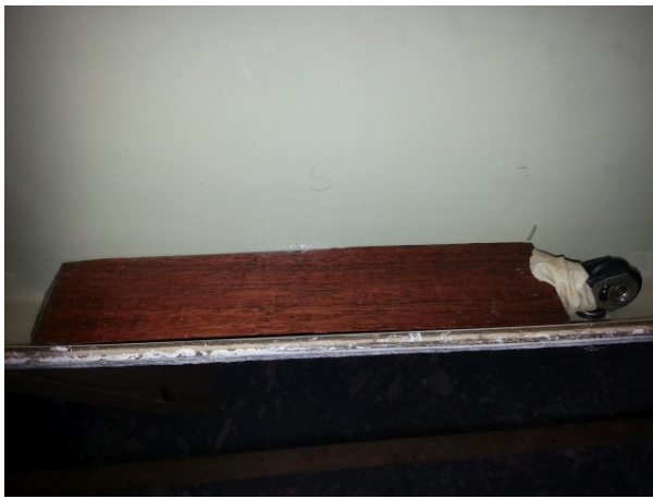
Figure 15: Mahogany strips in place ready for bonding in with epoxy mixed with a filler. This one has a pulley built into it to take the trapeze elastic through a hole in the deck
