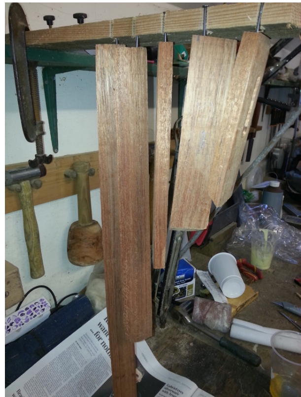
Figure 14: Mahogany pieces hanging up to allow epoxy to cure
