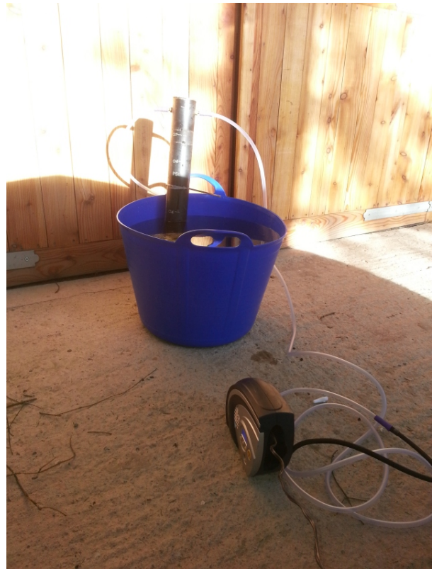
Figure 7: Makeshift tank pressure tester
