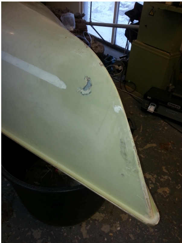
Figure 18: Defects prepared for Gelcoating in the bow
