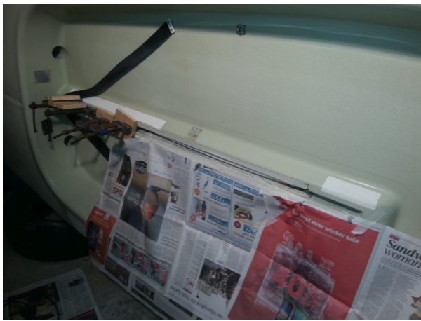
Figure 13: Whenever you use epoxy, make sure you cover the adjacent structures with newspaper and masking tape to ensure you don't spill epoxy where you don't want it.
