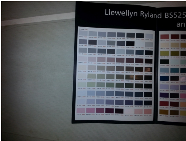
Figure 17: Once you choose your colour, you can order a pot of paste that allows you to mix at 1 to 10 ratio with gelcoat to give you your new colour.
