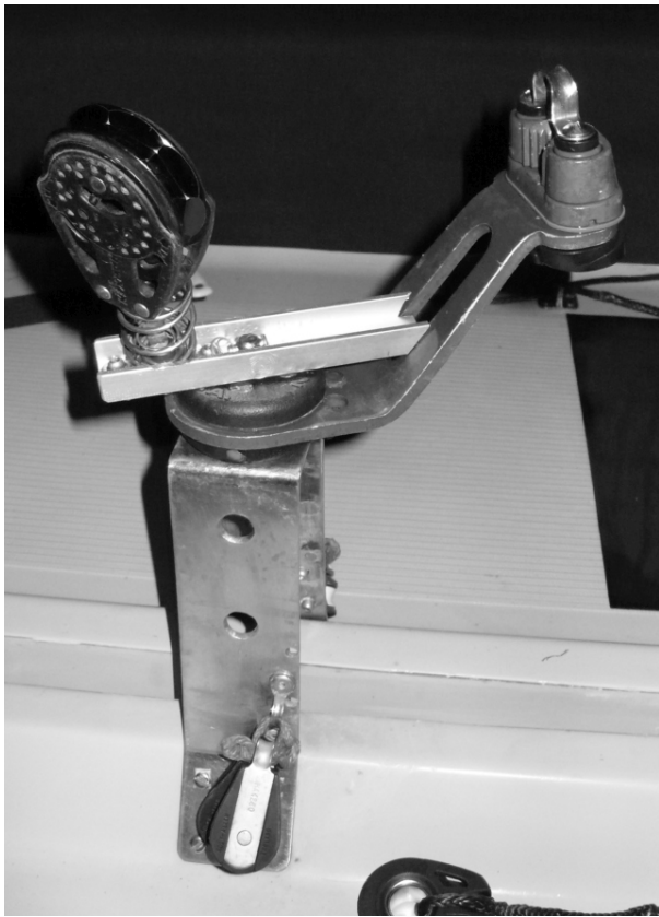
Figure 21: New mainsheet tower
